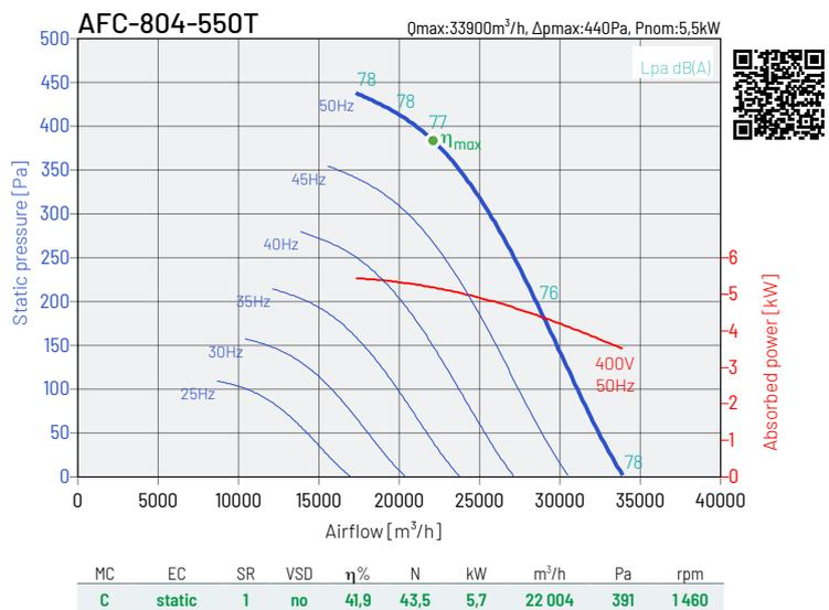
The performance characteristics of the fans are determined for a medium with a temperature of 20°C and atmospheric pressure of 1013.25hPa. Sound pressure level dB(A), determined at a distance of 1,5 m
